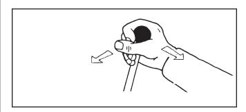
Loaders with 2-lever controls, ease both levers back to lift and rollback the bucket.
